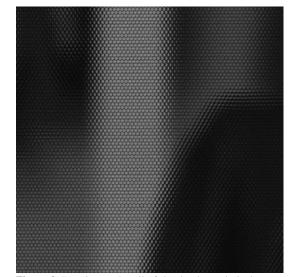
Figure 3. Raw image. Detail of the density and pixel structure on LFC (light field cameras).
