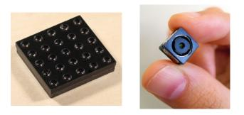
**Figure 6.** Left detail of the microlenses from Pelican Imaging Corporation. Right . Taken from [11]. Toshiba miniature lightfield camera (LFC) module for smartphones and tablets. Taken from [12]
