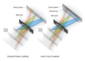
**Figure 4.** Microlenses galore. Comparison between a conventional camera (left) and the LFC (right). In the conventional camera the light from the focal plane (green)is the one focused in the image plane, the rest are out of focus points (blue and orange). The LFC proyected the 3 planes into a microlenses array that focused the image in the sensor plane therefore the out of focus image is digitally synthesized. Taken from [7]
